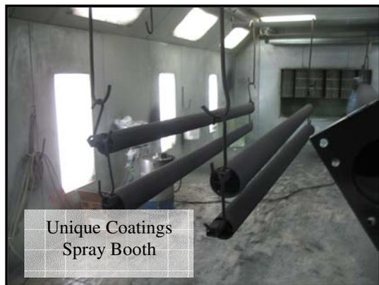
application of the finish coat. Finally, the finish coated pole is returned to the oven a third time to set the two coatings and the pole surface together.
