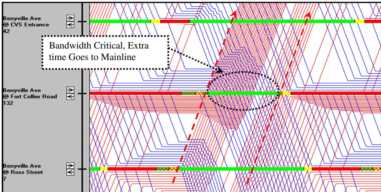
**Figure 4. Time-Space Diagram Illustrating where the Plan Force Mode was Used**
