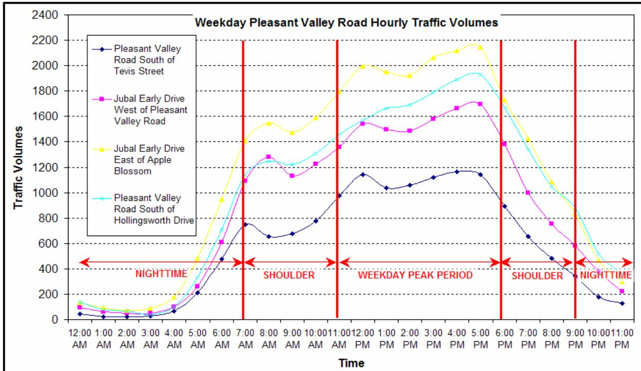
Figure 2. Traffic Volume Analysis to Identify Signal Pattern Start and End Times
